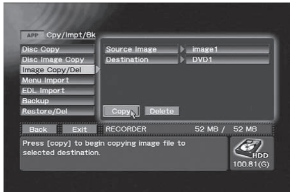
Using APP section → [Cpy/Impt/Bkup] → [Image Copy/Del] to create a disc from an image file
